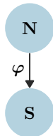
Figure 2.1: Probabilistic graphical model of a NeSy system. \mathbf{N} represents the subsymbolic state, while \mathbf{S} represents the symbolic state. The neural predicate \varphi maps the subsymbolic state to a probability distribution over the symbolic state.
